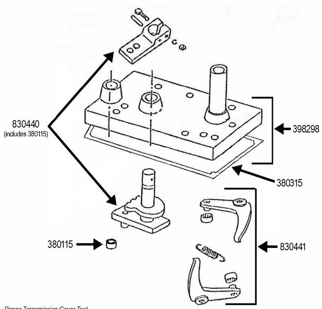
830430 - Range Transmission Cover Tool Removal and Installation Tool for 398298 Transmission Cover
