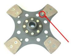
Care must be taken when replacing this type of clutch so that the loose PTO disc is correctly located to the engine's flywheel. The disc will remain loose after bolting the clutch to the flywheel. The PTO disc spline has a large leading edge to assist correct alignment during tractor reassembly.
